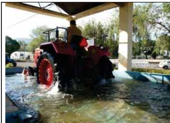
Water proofing test of tractor at CFMTTI, Budni
